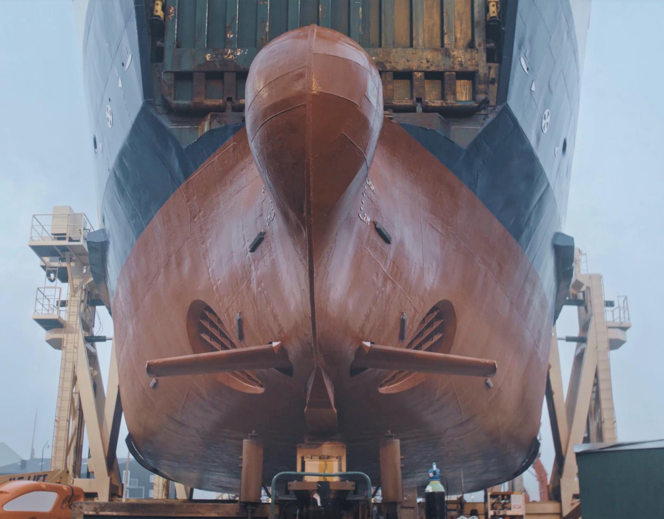
M/F Teistin with the bow foils deployed at MEST Shipyard in Tórshavn
