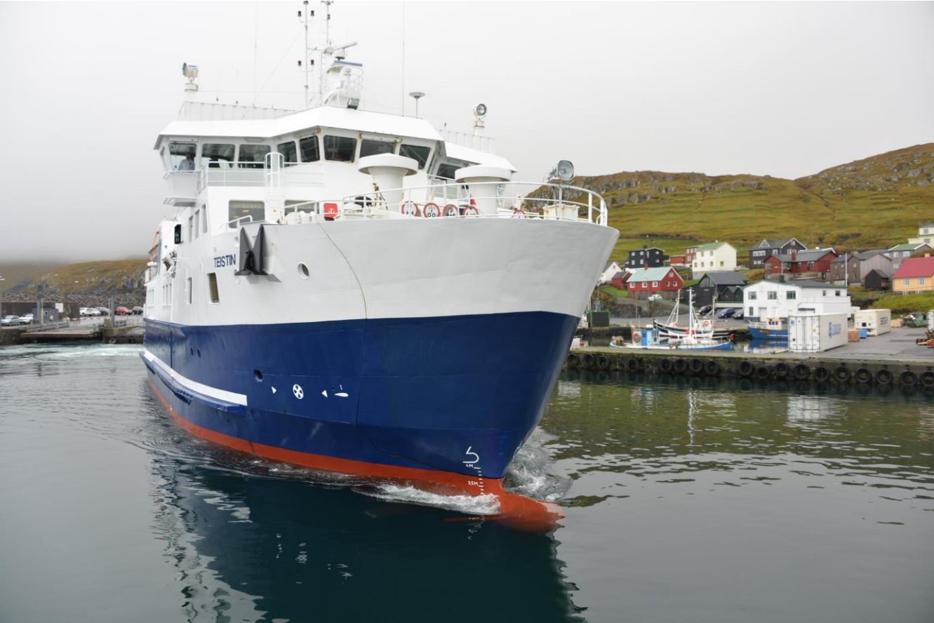
M/F Teistin on her way out of Skopun Harbour in the Faroe Islands with the foils deployed.
