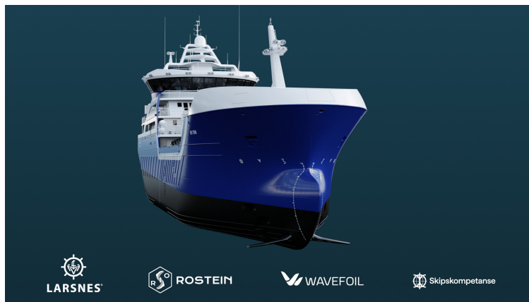
Figure 1: Ro Spirit with Wavefoil WF3970 bow foils installed.
